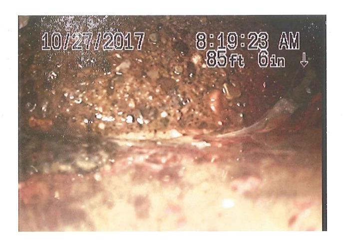
The above picture is a screen shot of the video at approximately 85 feet from the pool. This puts this obstruction at near the 90 degree fitting to the pool equipment room. You can see the rock and debris clogging the pipe. The camera was not able to get past this obstruction to finish the pipe run. This large amount of debris is only possible due to a large break in the pipe.
