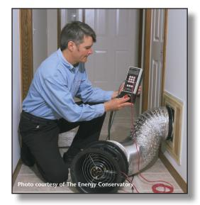
Did you know that testing ductwork in your house is now required by the Washington State Energy Code (WSEC) if you are repairing or replacing certain parts of your heating or cooling (HVAC) system?
