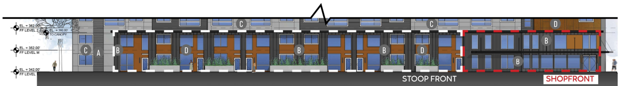
BUILDING A WEST ENLARGED ELEVATION-FLEX SPACE BUILDING TYPE WITH SHOPFRONT AND STOOPFRONT FRONTAGES 238 LINEAL FEET OF FRONTAGE | 31% TRANSPARENCY FOR SHOPFRONT FRONTAGE
