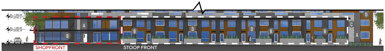
BUILDING B WEST ENLARGED ELEVATION-FLEX SPACE BUILDING TYPE WITH SHOPFRONT AND STOOPFRONT FRONTAGES 260 LINEAL FEET OF FRONTAGE | 31% TRANSPARENCY FOR SHOPFRONT FRONTAGE
