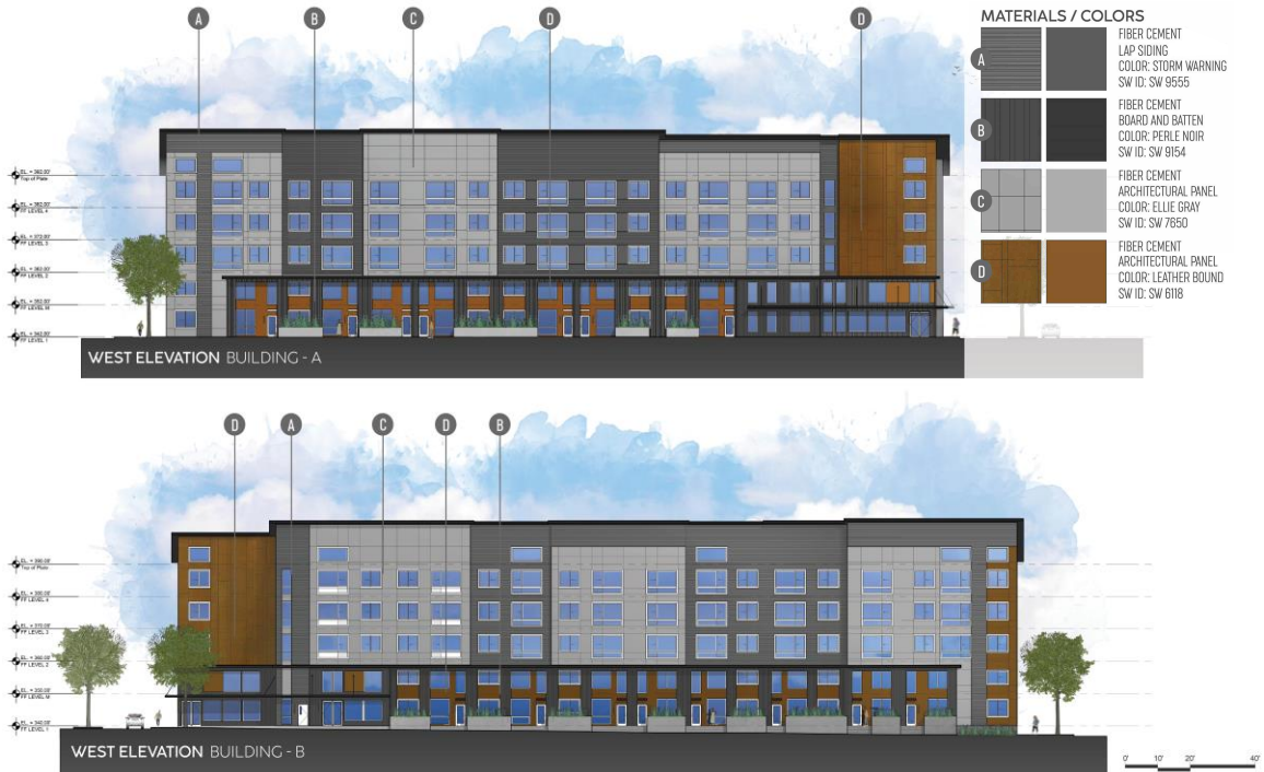
Exhibit 8. Exterior Elevations Buildings A & B.
